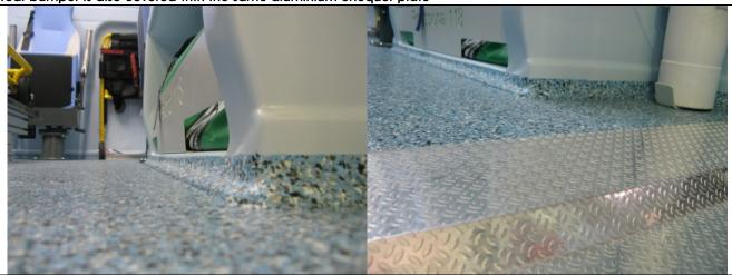
**ILLUMINATION OF THE AMBULANCE ACCESSES:** application of the aluminum profile with integrated blue led light under the rear bumper and on the edge of the lateral floor. The lights switch on and off with the opening and closing of the rear doors. (The electric step is not installed).
