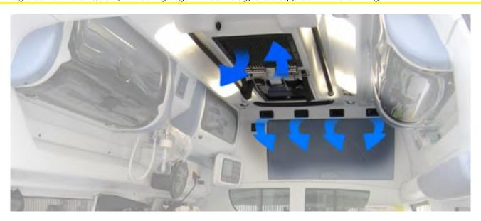
N. 1 AUTOMATIC AIR CONDITIONING SYSTEM with digital setting of the temperature, including an heating/cooling evaporator independent from the original system of the vehicle. It ensures inside the medical compartment the ideal micro-climate for the comfort of patients and operators.
